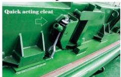
There are various ways to secure the hatch covers once they are in place, depending on the type. Modern covers may be self-cleating or secured by hydraulically operated cleats or wedges, but the most common type on older vessels is the manual quick-acting cleat, having a cam at the upper end, which is forced onto a snug on the hatch cover panels.
