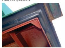
When leakages occur, the rubber gaskets of the hatch covers are usually hard, deeply and permanently compressed, chafed or loose, and may even have sections missing. Gaskets may be of solid rubber, or have a hollow or sponge core.
