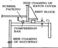
The compression bars on hatch cover panels and on hatch coaming tops need to be straight and the top edge must be well rounded and have an even surface. The compression bar consists of a stainless steel bar, welded to the top of a supporting flat steel. Such compression bars must always stay smooth and even.
